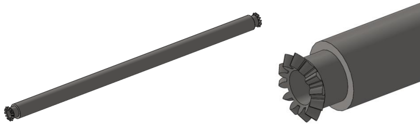
Fig.31. The mechanical element that distributes the movement between the two groups of penetrating screws (double pinion).
