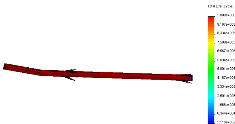
Fig.24. Total life diagram for the analyzed system of the nail with fixing arms actuated by a planar mechanism with bars.
