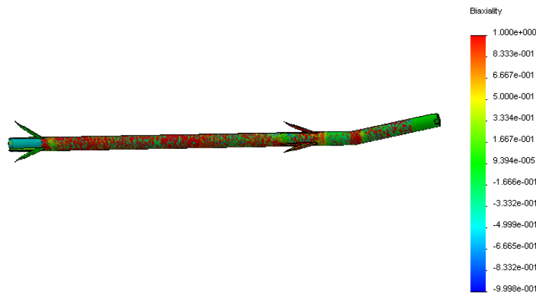
Fig.14. Diagram of the biaxiality indicator for the analyzed system of the nail with fixing arms actuated by a rack and pinion mechanism.
