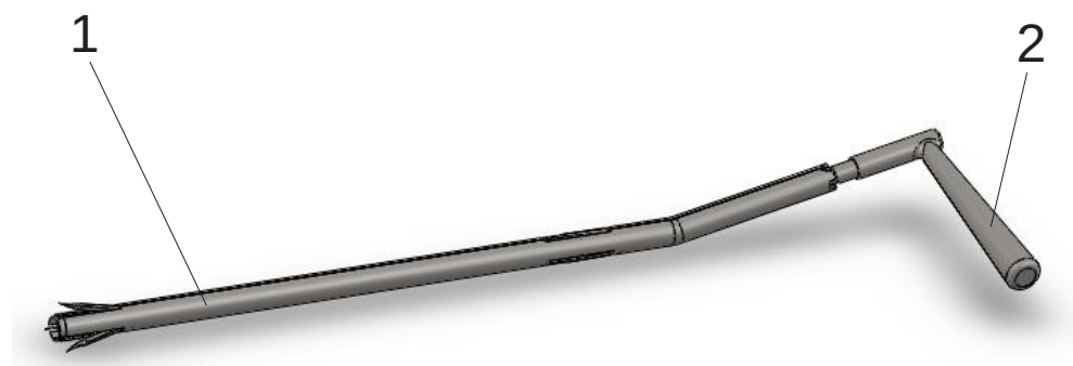
Fig.1. The model of the nail with gear-rack mechanism: 1- the body of the nail with the mechanisms; 2-actuation key.
