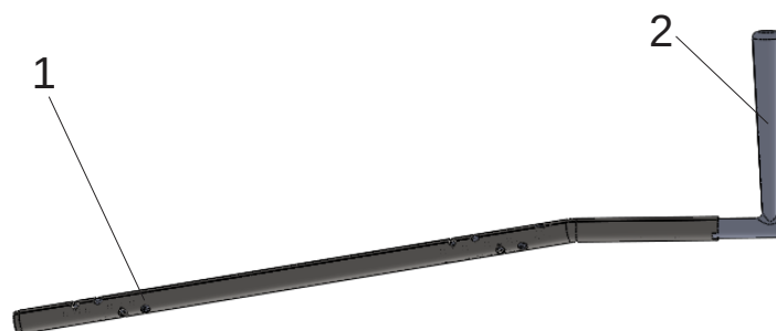
Fig.27. The model of the nail with gear-rack mechanism: 1- the body of the nail with the mechanisms; 2-actuation key.
