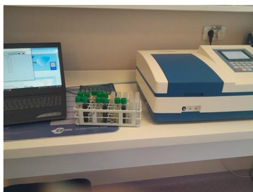
Figure 5. Determination of total polyphenols by UV-Vis spectrophotometry
