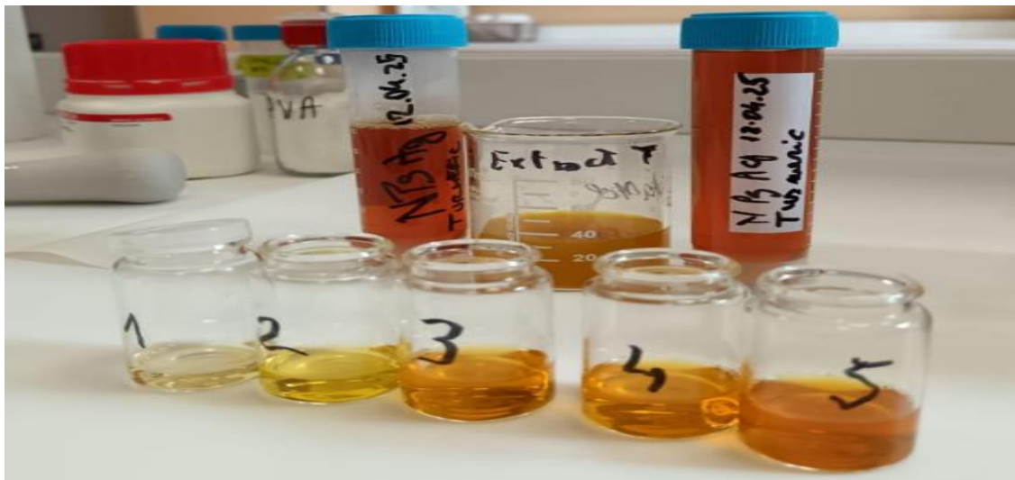
Figure 2. Samples numbered 1–5 obtained after the reaction between turmeric extract and \text{AgNO}_3 . The color intensity varies depending on the efficiency of Ag nanoparticle synthesis.
