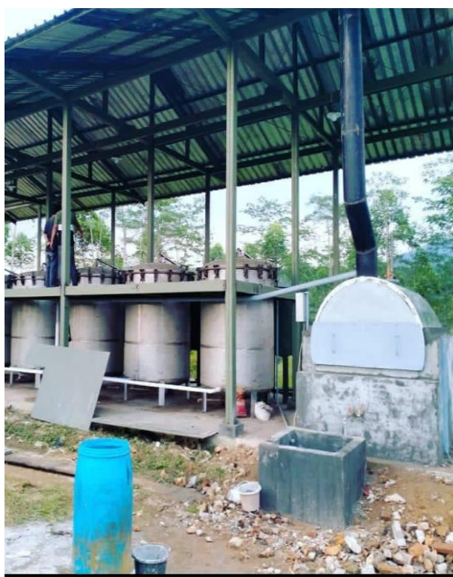
Figure 1. Modified essential oil distillation equipment model 1 heating boiler (Capacity 2 000 Lt) with 4 distilling kettles (Max capacity 500 kg/distilling kettle)
